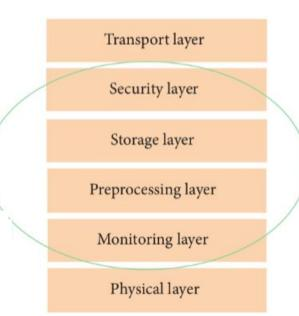
Monitoring and pre-procesing are carried out at the edge, before sending data to the cloud
